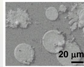
*Layered and graded architectures through successive splat quenching*
