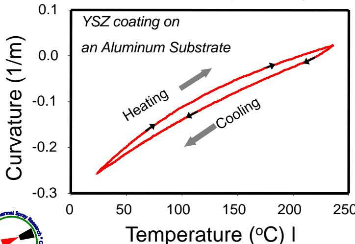
After spraying, the coating (with substrate) is heated inside a furnace. The temperature change induces mismatch strain, and the curvature of coating changes. The continuous recording of one thermal cycle provides an ANELASTIC curv-temp plot, which is then converted to a stress strain curve to quantify the coating compliance.
