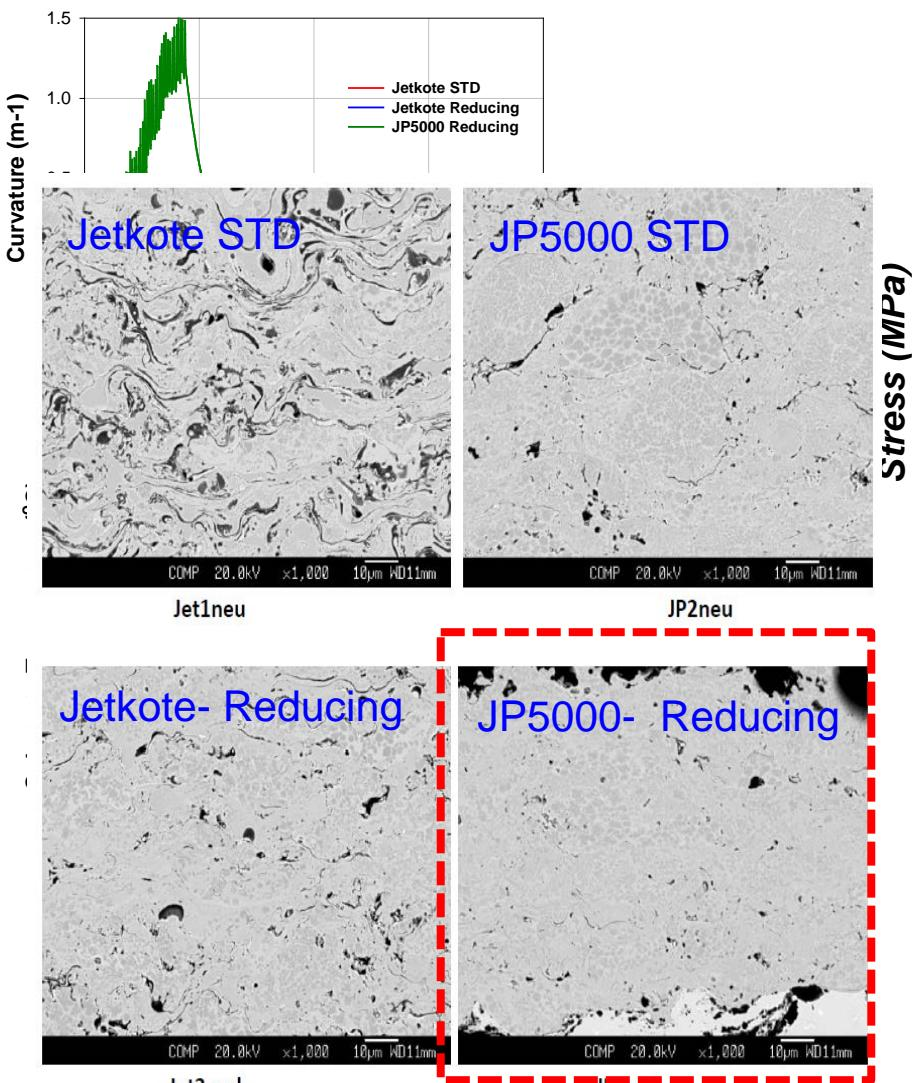
**JP5000 chosen due to microstructure and compressive stress state.**
