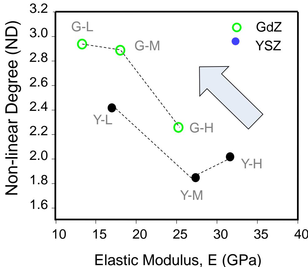
*A systematic shift in  $\text{Gd}_2\text{ZrO}_7$  from YSZ for the given set of parameters*
