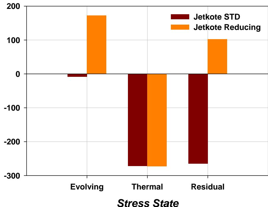
*HVOF process type and spray conditions significantly affect deposition stresses and final stress state of the coating.*
